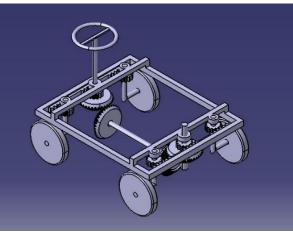
gear thus steering control will get transferred to all the four wheels of the vehicle to turn the vehicle at 90<sup>0</sup>. During this operation when steering wheel will move in anti-clock wise direction it will result in anti-clockwise rotatio-
